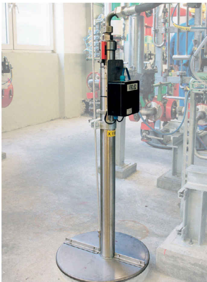
Lance system - moved hydraulically/pneumatically actuated
