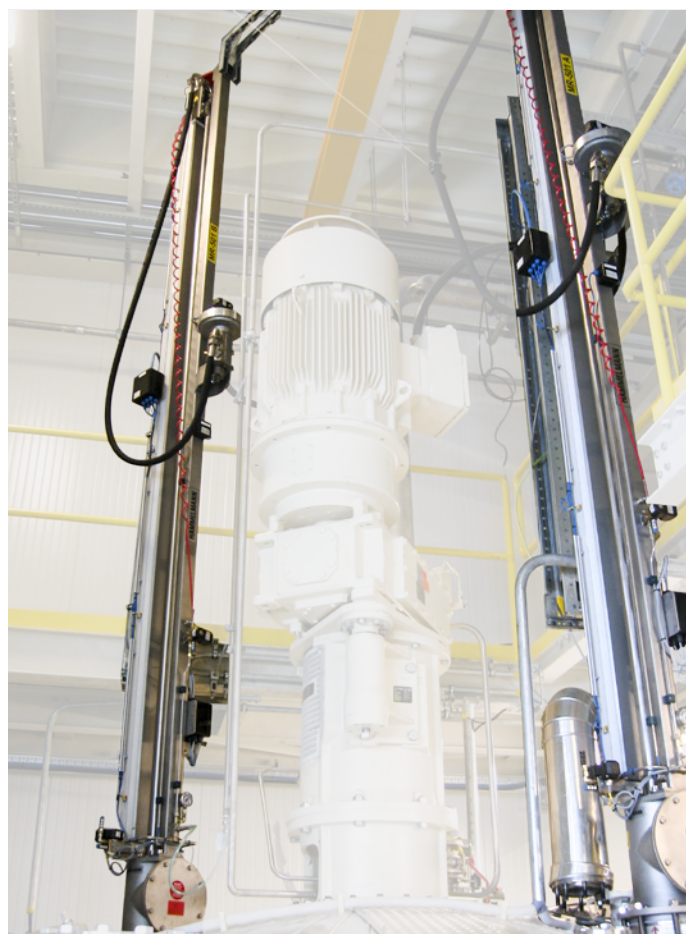
Lance system - moved pneumatically actuated
