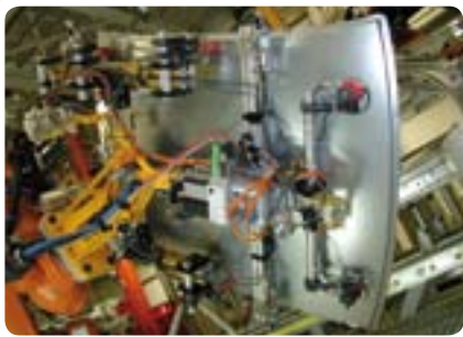
The Magnetic Gripper with vacuum handles a BMW car roof, but is also suitable for perforated steel plates, aluminium or stainless steel. Without change over!
