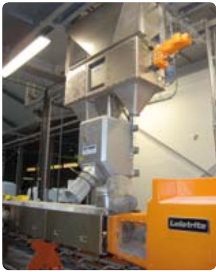
A metal detector in combination with a clean flow magnet. Ensures the removal of all metallic particles.
