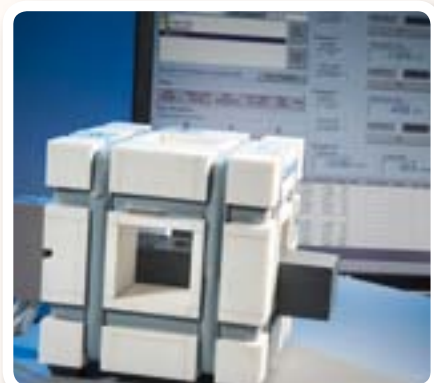
Goudsmit Supplies has a 3D Helmholtz coil, that can be used to measure the magnetization angle.
