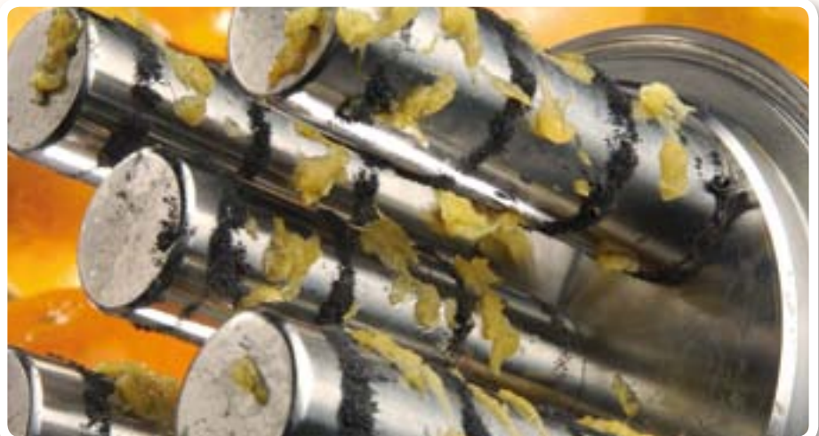
Magnet filter for the removal of iron particles from fruit pulp.
